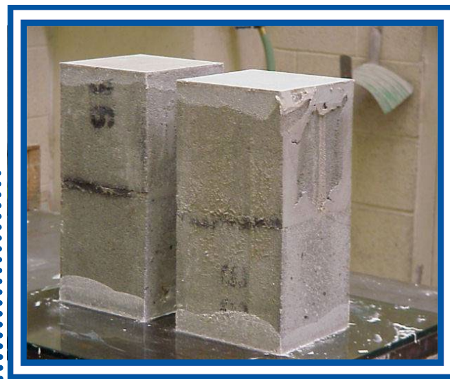
Figure 3: Concrete Masonry Prisms Capped and Ready for Testing
