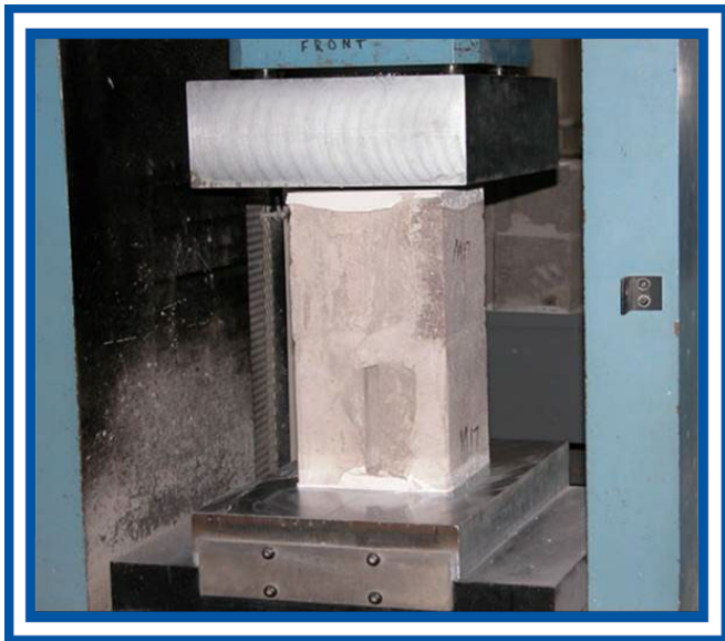
Figure 2: Compression Testing a Concrete Masonry Prism
