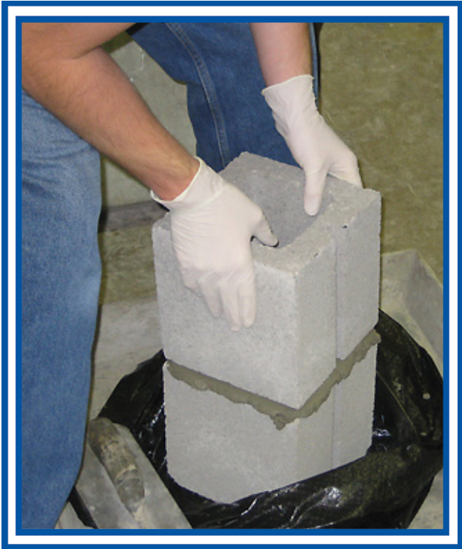
Figure 1: Preparing a Concrete Masonry Prism
