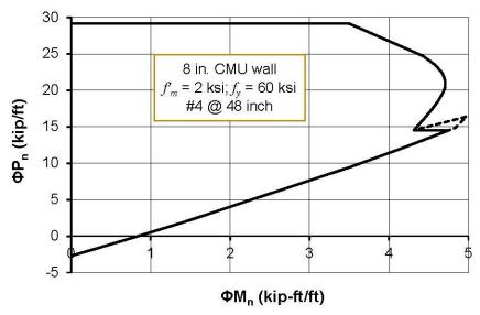
With the adoption of compression-controlled sections, the maximum reinforcement restrictions were removed except for intermediate and special reinforced masonry shear walls under in-plane loads, and for beams. These changes are covered below under the appropriate section.
