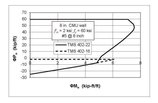
Section 9.1.4.4.2 can be confusing on first reading. For partially grouted walls under out-of-plane loading there can be strange behavior in the transition region, as shown below by the dashed line. The nominal capacity is increasing at a slower rate than the decrease in the strength-reduction factor. Section 9.1.4.4.2 is saying the solid line needs to be used for the interaction diagram and not the dashed line.
