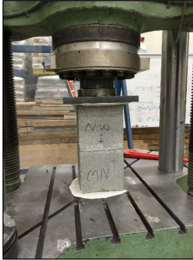
Figure 24. Test Setup for Grout and Masonry Prisms
