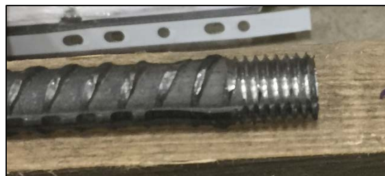
Figure 7. Typical Upset Threads
