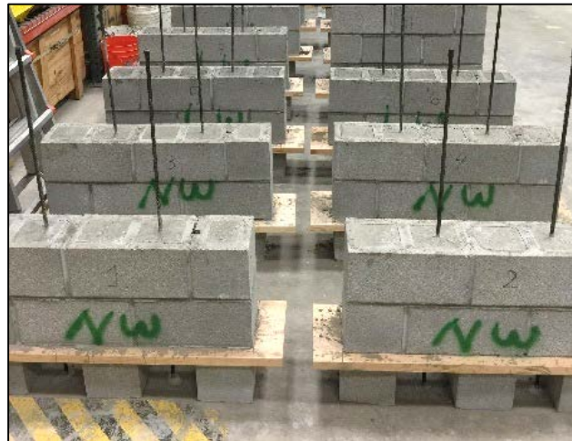
Figure 21. Completed Wallettes Prior to Testing
