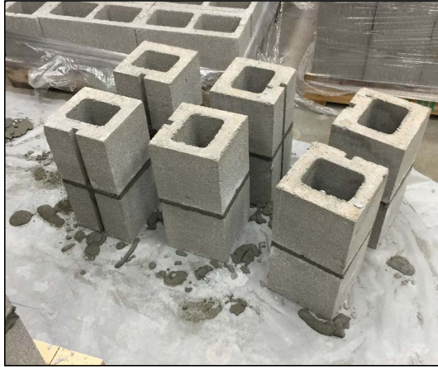
Figure 11. Masonry Prisms Prior to Grouting
