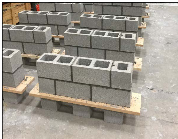
Figure 12. Wallettes Prior to Grouting
