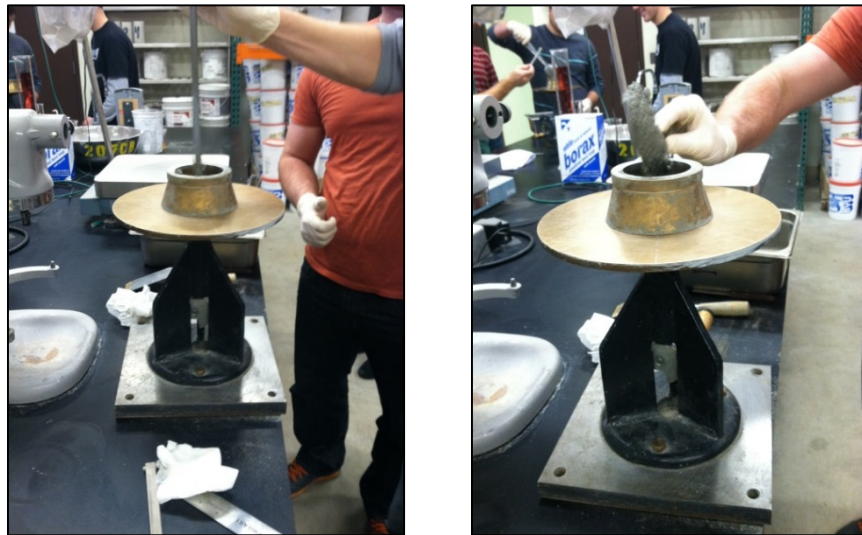
Figure 22. Mortar Flow Tests
