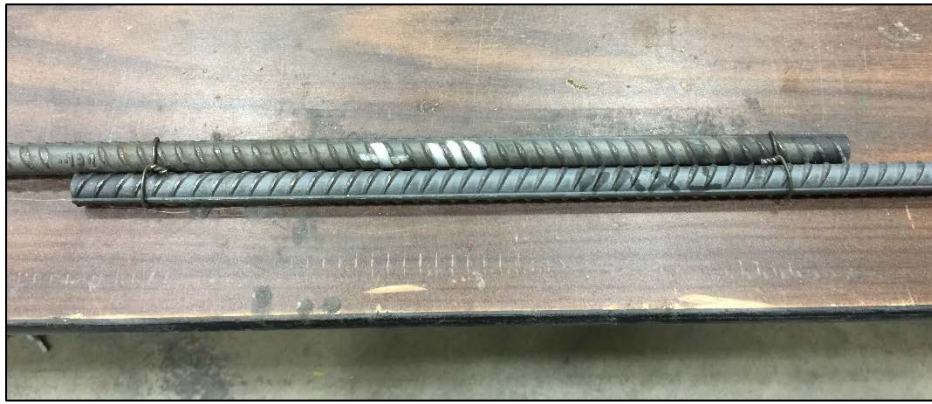
Figure 14. Typical Reinforcement Splice
