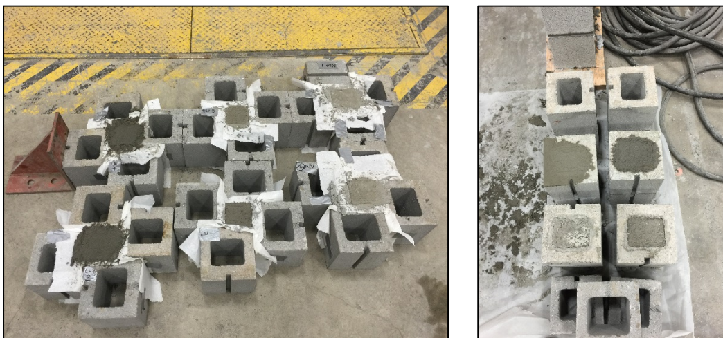
Figure 20. Grout and Masonry Prisms
