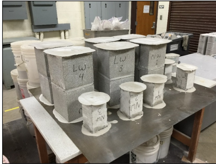
Figure 23. Capping of Grout and Masonry Prisms
