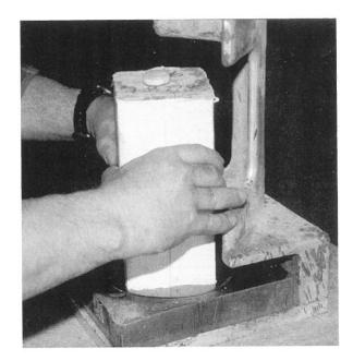
Figure 29 Capping the Grout Sample
