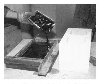
Figure 14 Pouring Sulfur Capping Material
