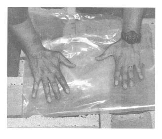
Figure 26 Protecting the Grout Sample
