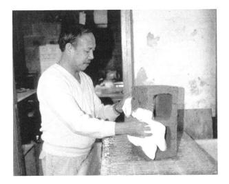
Figure 4 Removing Visible Surface Water
