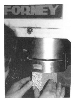
Figure 10 Compression Testing a Coupon
