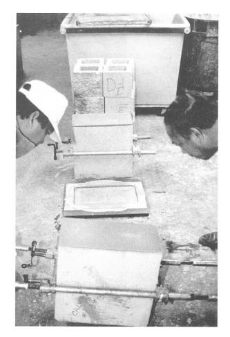
Figure 21 Moving a Prism
