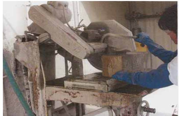
Figure 4: Saw-Cutting of Grout Specimens from Concrete Masonry Unit
