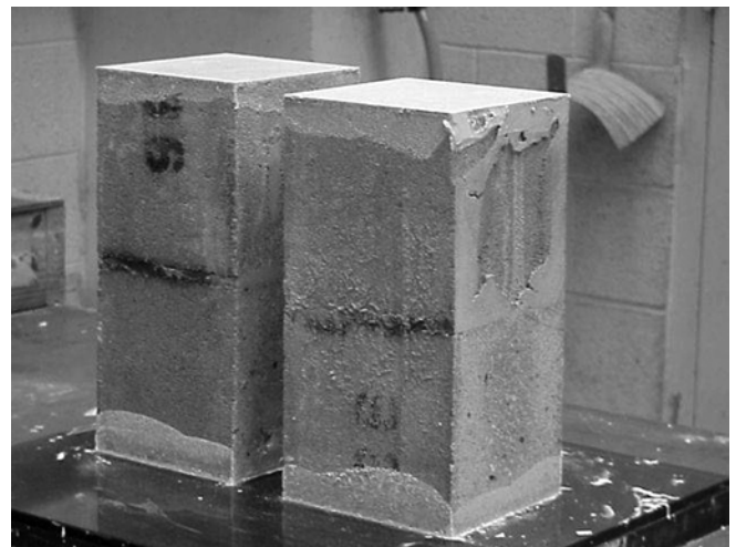
Figure 3: Concrete Masonry Prisms Capped and Ready for Testing
