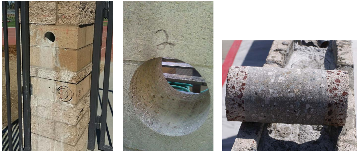
Figure 3. Illustration of the Destructive Nature of Coring
