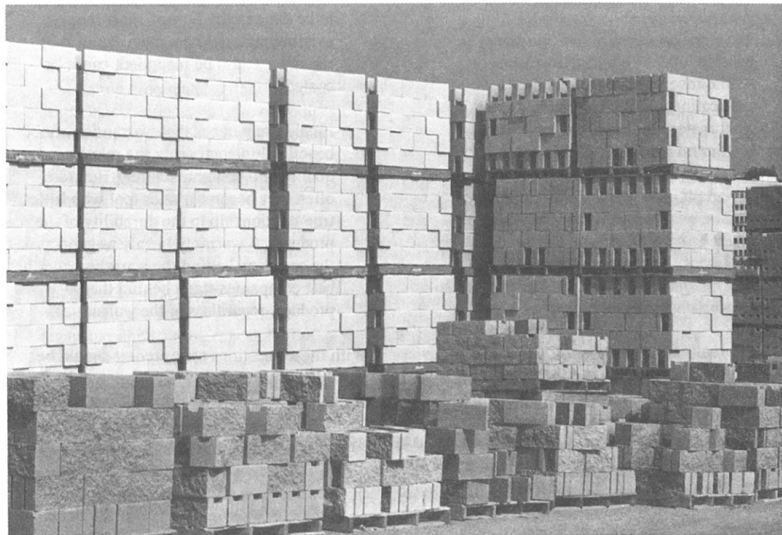
Variety of concrete masonry units at a manufacturing plant.
