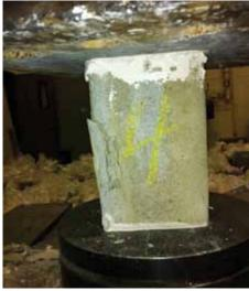
Figure 3: Grout samples during testing.
