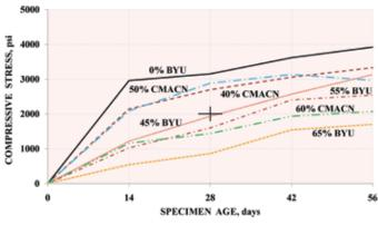
Figure 4: Grout strength – fly ash replacement set.
