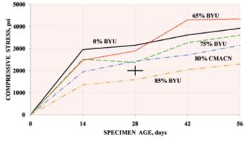
Figure 5: Grout strength – fly ash-GGBFS replacement set.
